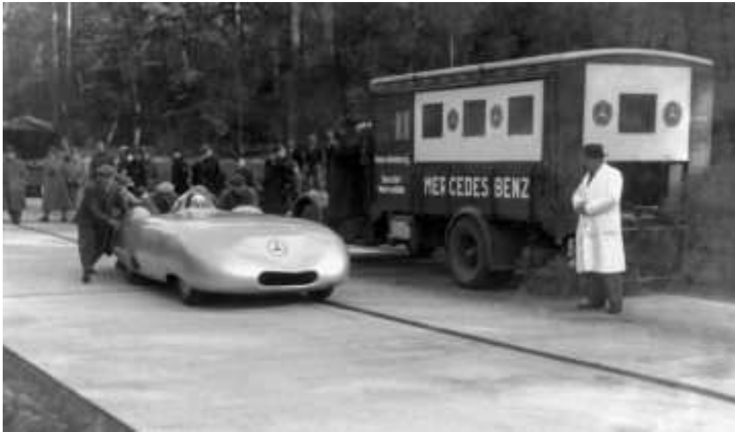
Caracciola gets a push in the 1936 speed record car. Note the large dent in the nose panel caused by air pressure on the thin aluminum skin during a previous run.
